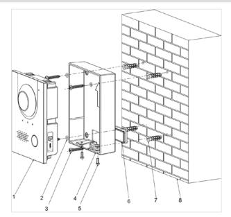
**Step1** With the help of installation diagram, hammer four expansion screws into the wall.
