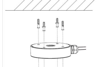
Route the cables through the cable hole (take side conduit cabling for example) and connect the cables. Then fasten the camera onto the junction box with screws.
