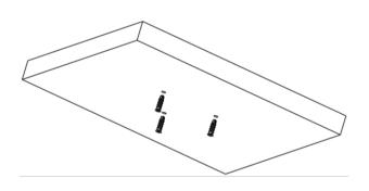
3. Install the sponge and the rubber plug respectively to the mounting base.
