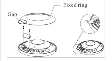
8. Install the cover of microSD card slot and then fasten the camera onto the bracket with screws.
