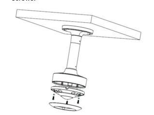
9. Install the fixed ring back to the camera and then fix the bracket with screws.
