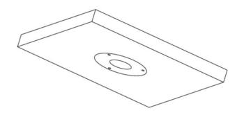
2. Tear off the drill template and insert the plastic plugs.
