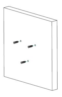
5. Fix the mounting base to the wall with the screws provided.
