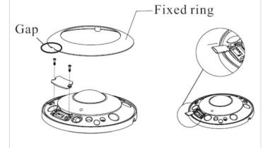
8. Install the cover of the microSD card slot and then fasten the camera onto the bracket with screws.
