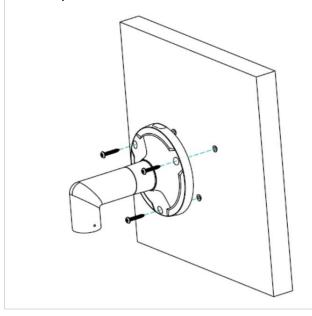
6. Mount the water-proof ring to ③, and then screw ③ with the water-proof ring into ⓒ.
