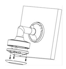
9. Install the fixed ring back to the camera and then fix the bracket with screws.
