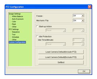
To restore default settings to all the settings in PTZ Configuration, click Load Camera Default (Include PTZ). To restore default settings to Image Settings and System Configuration settings only, click Load Camera Default (Exclude PTZ).
